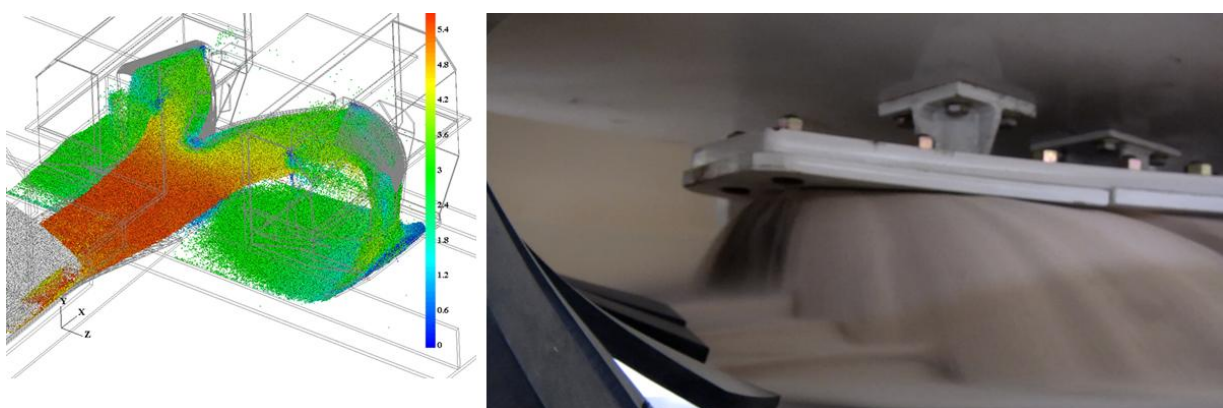
Figure 11: Mobile Offload DEM showing the parabolic plough and twin discharge hoods.
