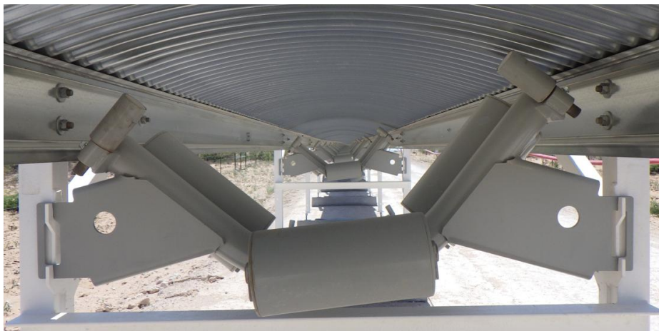
Figure 6: Special Idler Frame Transom design used in conjunction with the Ninja Idler change system
