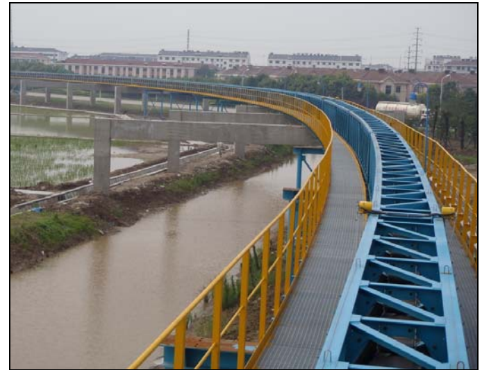
Figure 8. 350mm diameter ST2000 EPDM heat resistant pipe belt, with material temperature 180°C.
