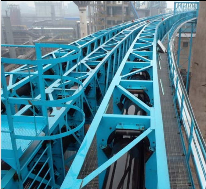
Figure 9. Two parallel 300mm diameter heat resistant Confine fabric pipe belts and a 400mm diameter Confine fabric pipe belt.
