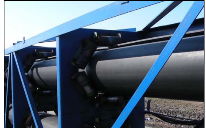
Figure 7. 400mm diameter ST1100 Low Rolling Resistance Pipe Belt.
